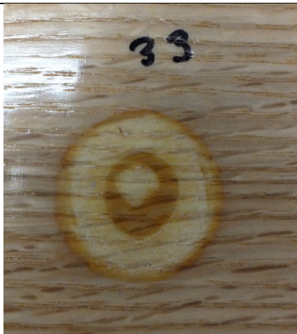
33, Nitric Acid, 70%, Erosion of coating
