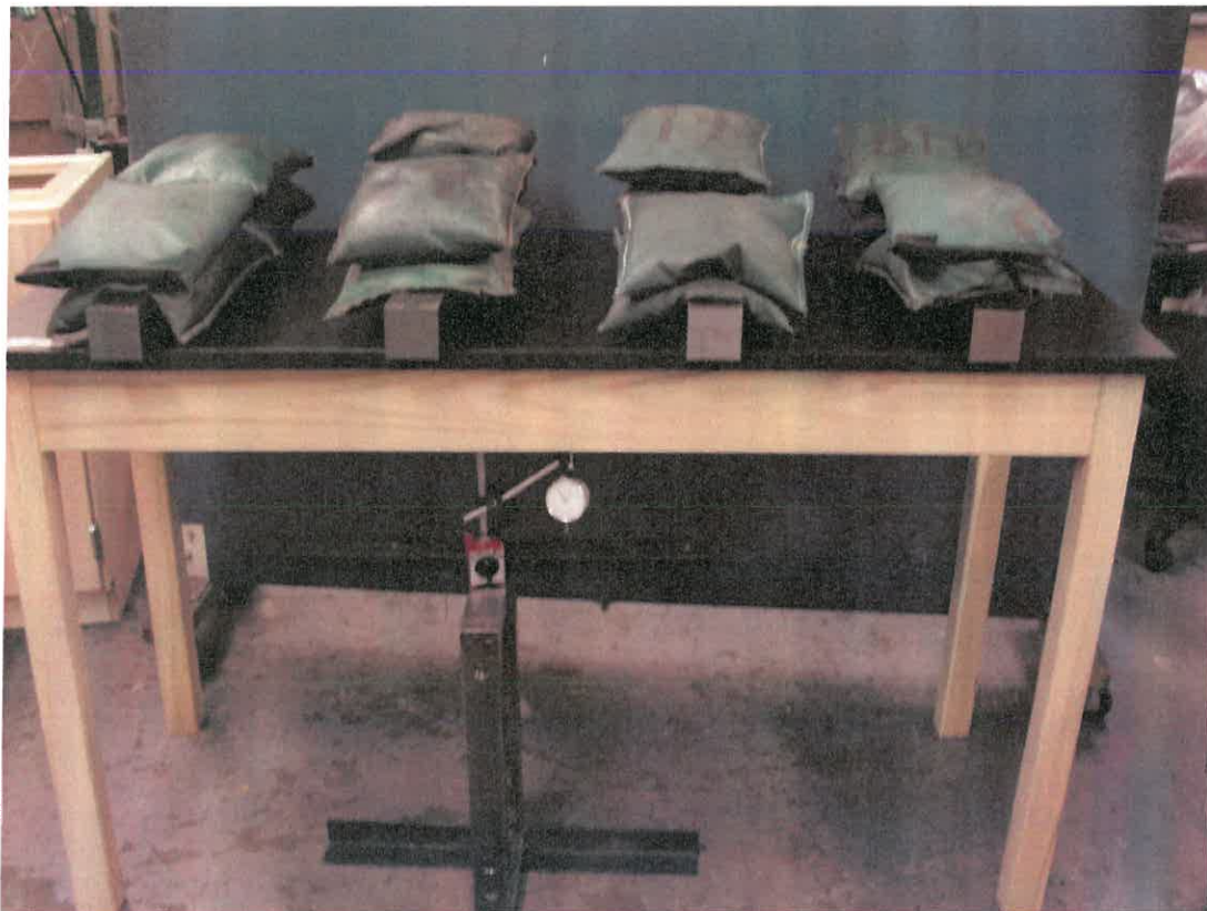
Figure 1. 10.2 Table Static Load Test; Plywood Frame
