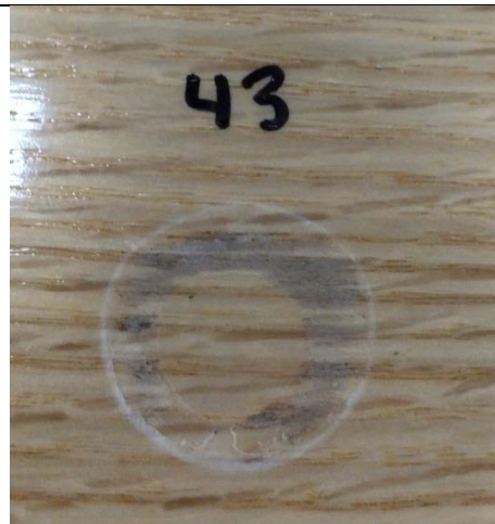
43, Sulfuric Acid 77%, Erosion of coating/pitting
