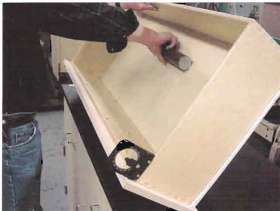
Figure 12. 6.4 Cabinet Drawer Internal Rolling Test; Setup
