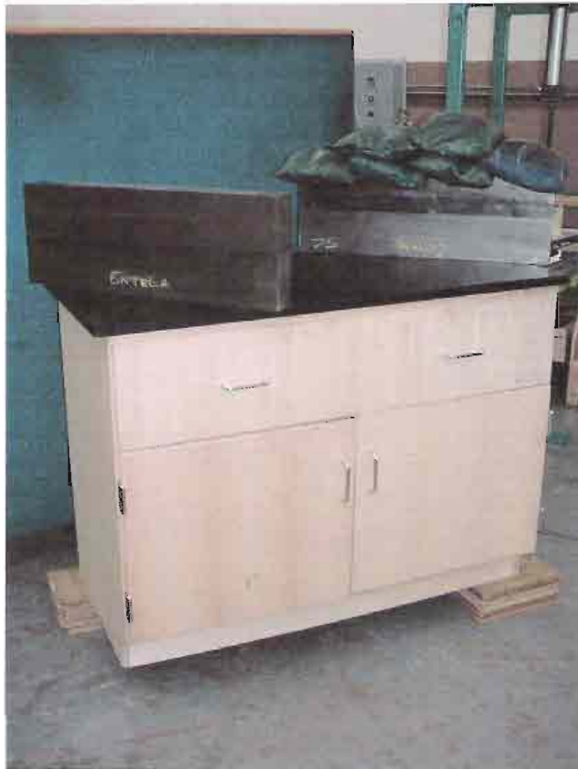
Figure 3. 4.4 Cabinet Torsion Test
