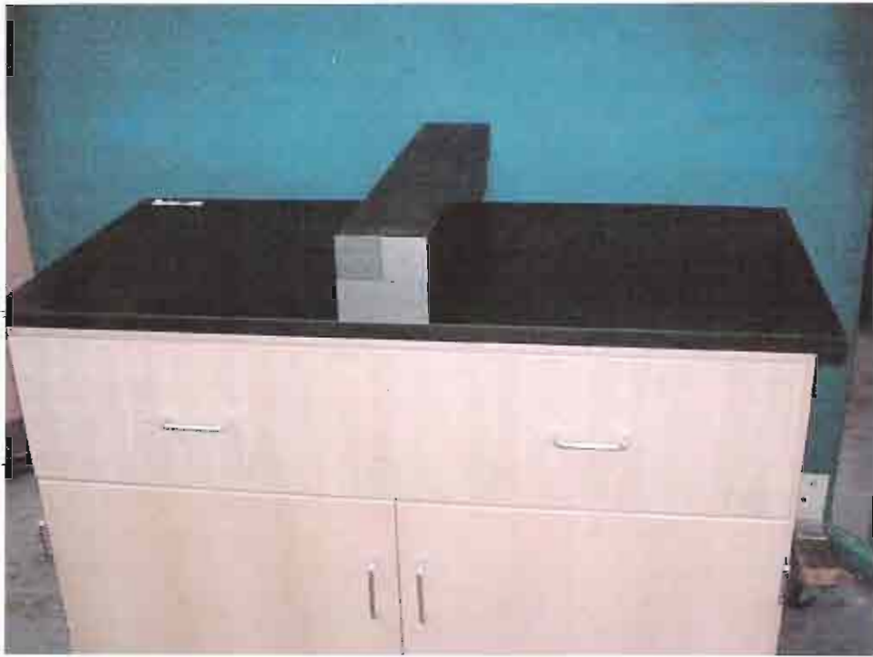
Figure 2. 4.3 Cabinet Concentrated Load Test
