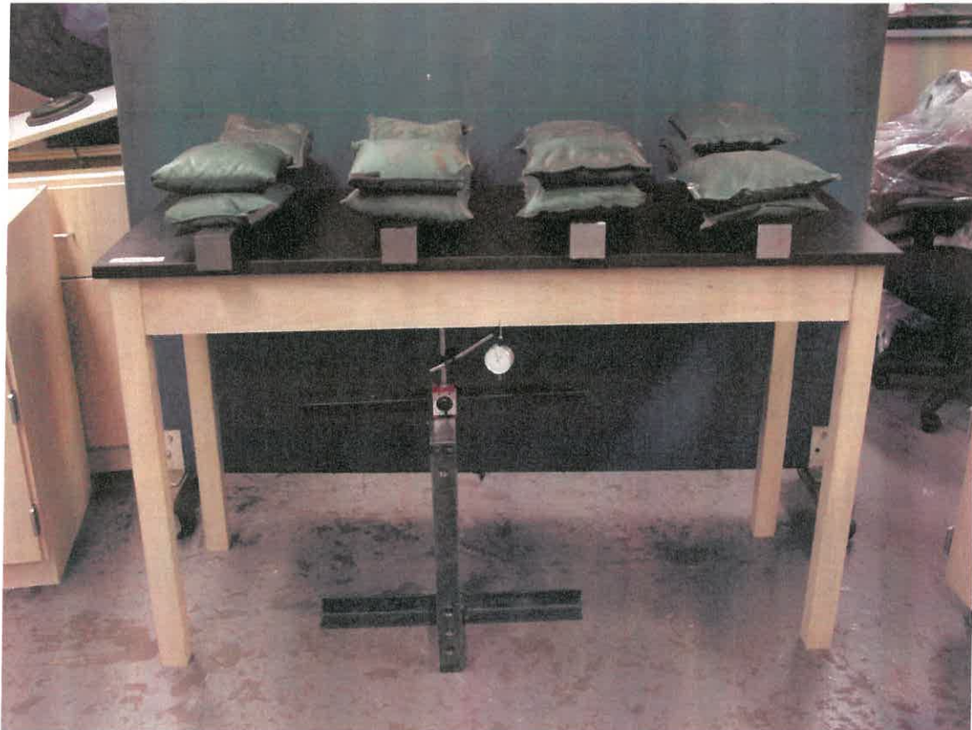
Figure 2. 10.2 Table Static Load Test; Solid Wood Frame
